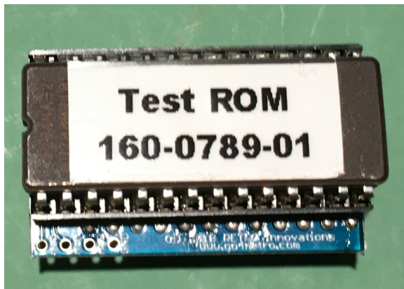
Test EPROM in Adapter
